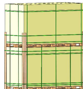
Short-side vertical package(some modules use presswood pallets, the illustration shows the full
