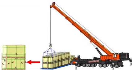
Vertical landscape package unloading with crane
