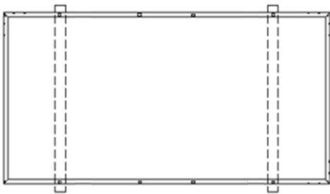
Fig. 3 Bolt installation for 60cell
