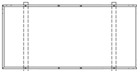
Fig. 4 Bolt installation for 66cell
