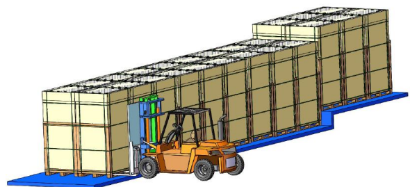
Long-side vertical package unloading with forklift
